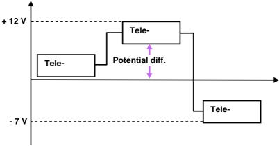
Fig. 4: Potential shift at signals
