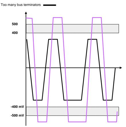
Fig. 12: PROFIBUS MBP (PA) with defective bus terminator
