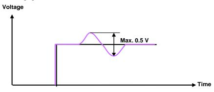
Fig. 8: Signal waveform for non-connected PROFIBUS stations
