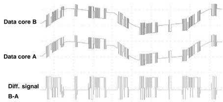
Fig. 6: Measurement PROFIBUS RS-485
