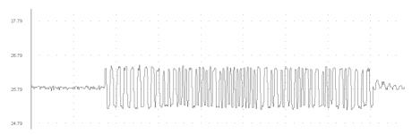
Fig. 13: Measurement PROFIBUS MBP (PA) (1 telegram)
