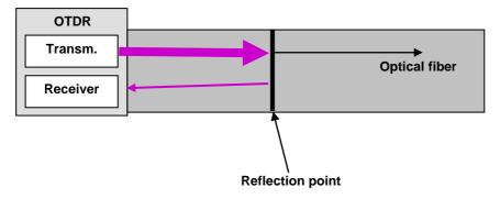
Fig. 2: OTDR measurement principle
