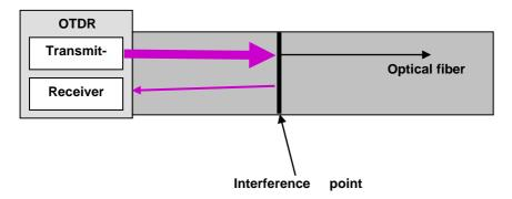
Fig. 14: OTDR measurement principle
