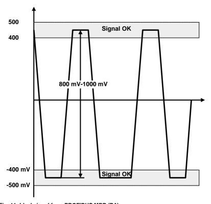
Fig. 11: Ideal signal form PROFIBUS MBP (PA)
