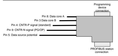
Fig. 3: Measurement plug oscilloscope measurement
