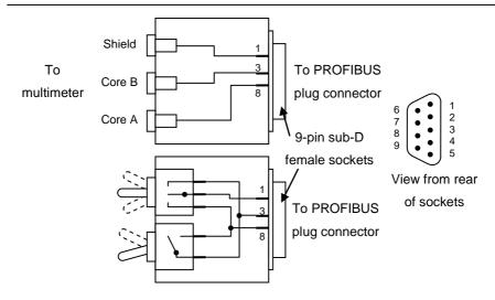
Fig. 16: Measurement aid sockets (PROFIBUS RS485)
