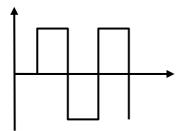
Overlaid signal (original signal + reflection) for too little terminating resistance
