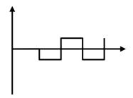
Overlaid signal (original signal + reflection) for too much switched-on terminator resistance
