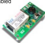
direct data access and control via standard web browsers. Configuration files are stored in XML format and can be transferred to/from a PC using FTP. Configuration files can also be viewed and edited via standard text editors, XML editors and web browsers. As new firmware becomes available, the unit can be upgraded.
